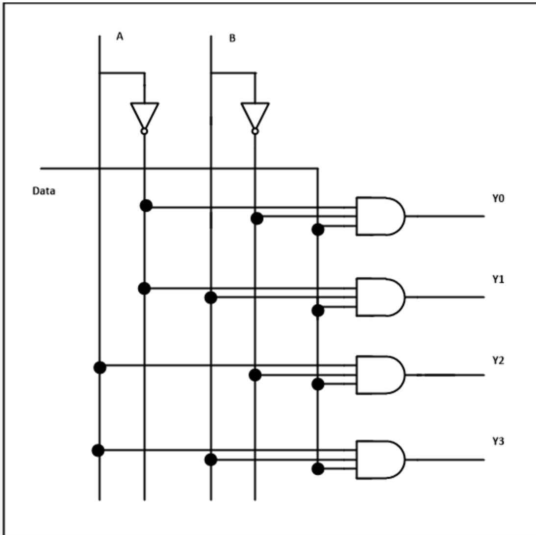
1 to 4 Demultiplexer Circuit Diagram – [ElectronicsHub.Org](http://www.ElectronicsHub.Org)
