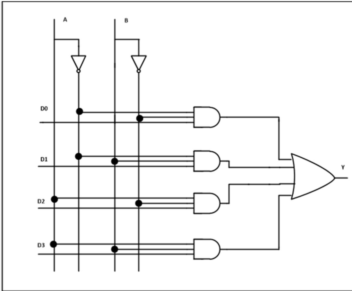
4 to 1 Multiplexer Circuit Diagram – [ElectronicsHub.Org](http://ElectronicsHub.Org)
